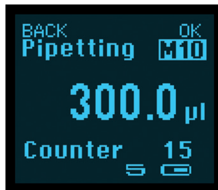
M10 indicates that 300 µl pipetting has been saved on memory place 10.
