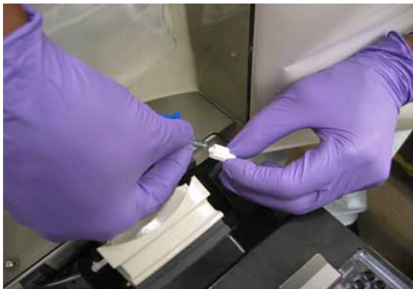
Figure 6-13 – Connect ID Broth Solution to Dispense Tubing Set
