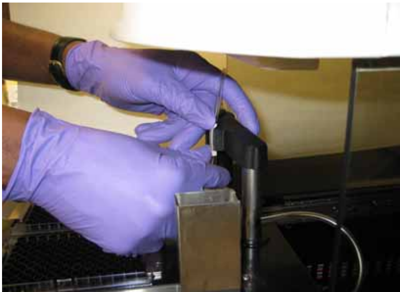
Figure 6-9 – Inserting Tube on Dispense Arm
