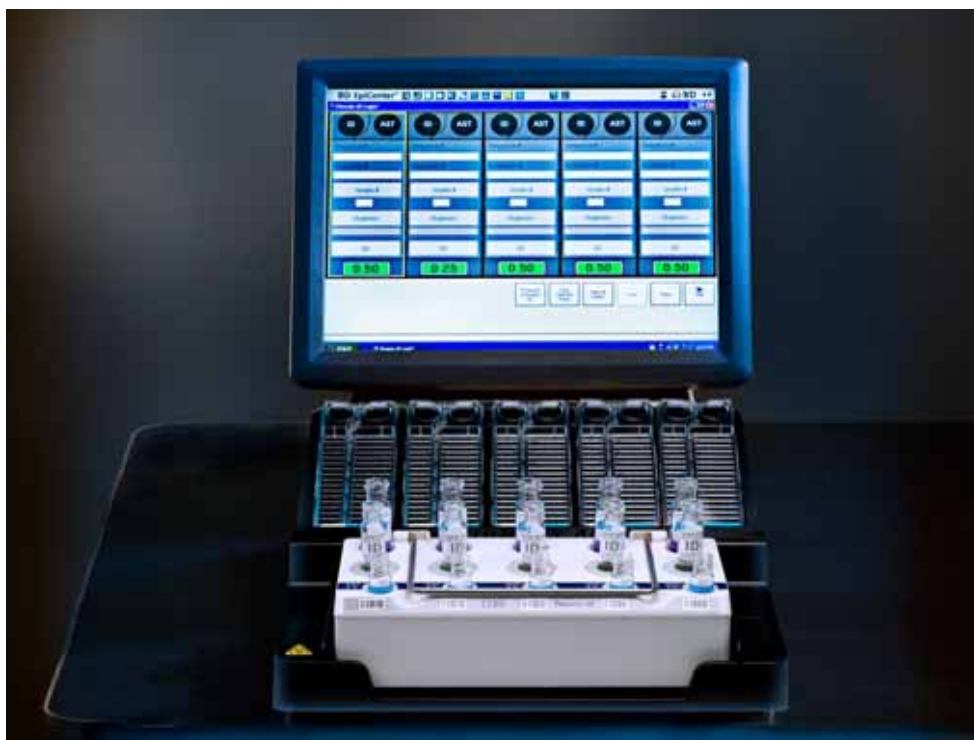
Figure 4-9 – Sample Rack in BD Phoenix AP Inoculation Station at BD EpiCenter Workstation
