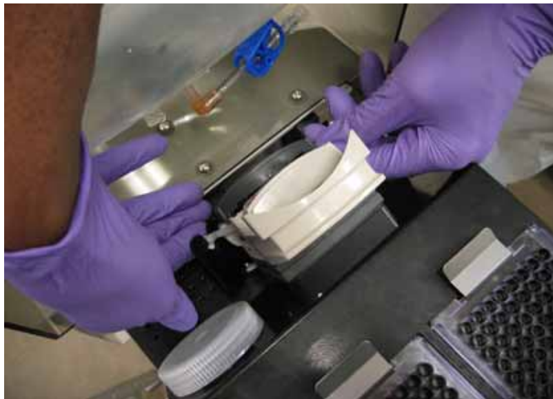
Figure 6-12 – Inserting Dispense Tubing Set Locators
