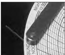
Chart recorder stylus and time line groove
