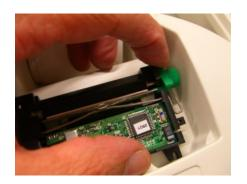
1) Press the green lever down as in picture below to lift the printing head
