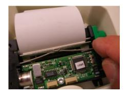
4) Align the paper and press the green lever back as in the picture.
